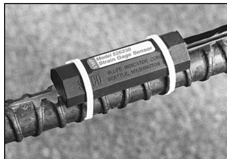
Spot-weldable strain gauge installed on reinforcing bar. The gauge is later waterproofed with mastic and tape.
