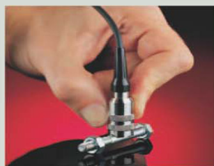
...and for measuring galvanizing, plating, anodizing and more.
