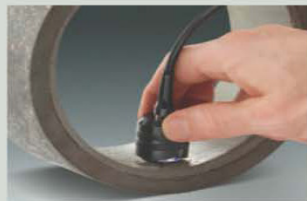
High-Range Probes for thick coatings, e.g. fire proofing, tank linings, etc.
