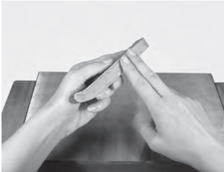
Fig. 6.01 Application of coupling paste
