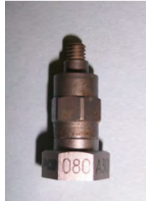
Accelerometer (with magnetic base)
