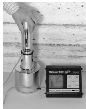
Fig. 6.1 Performance check of the concrete test hammer
