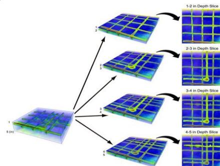
Collecting a grid of line scan results using the grid maps creates a data cube or 3D volume that can be visualized as a series of 25 mm thick depth slices or as a solid.
