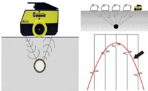
The system can scan concrete to depths of up to 0.5m where a cover meter would be limited to 150-200mm. The system is simple to use and only requires one operator. It is the choice of equipment for locating services, Post Tensioning and rebar.
