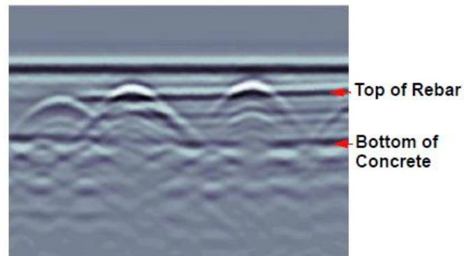
The image above shows three rebar at varying heights as well and the bottom of the concrete which is also reflects the radar signal.
