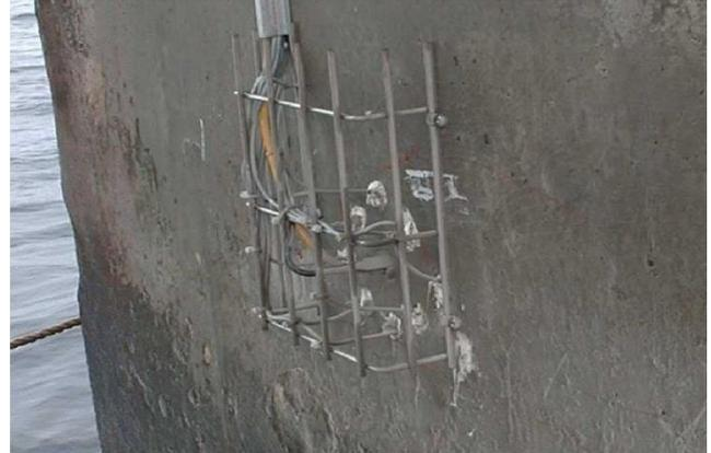
Figure 2. CorroRisk mounted on bridge pillar and covered with latticework
