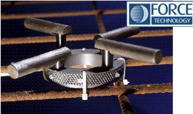
Figure 1 – Photo of CorroWatch Probe Installed
