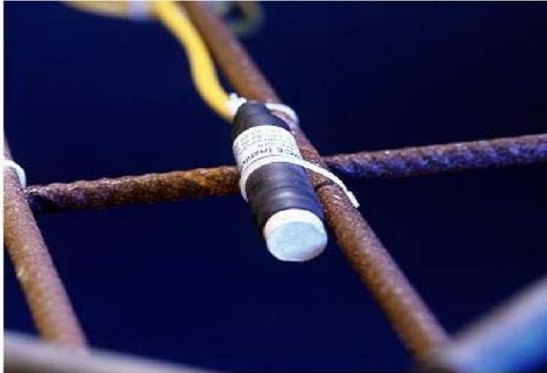
*The ERE 20 attached to the reinforcement*
