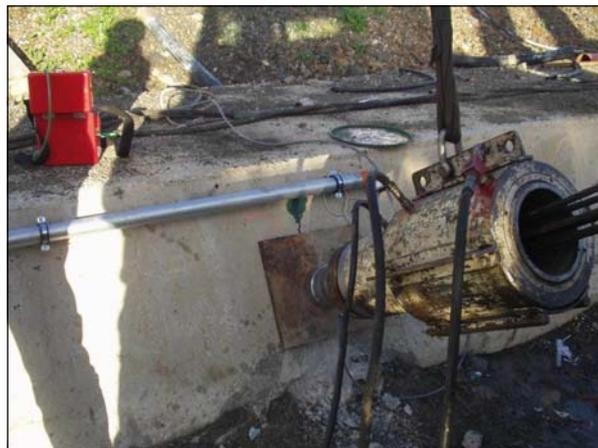
6. Place pressure jack onto top of cell and carry out the necessary tests recording the outputs and checking what load is being applied (see DATA HANDLING).
