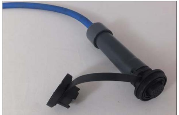
The VW-2106 contains an internal multiplexer allowing it to be connected to multi-channel instruments through its *Expansion* connector. Appendix B – Expansion Connector Pin-out provides the pin-out of this connector. Mating halves of the connectors are available from Geosense if your current sensors are not equipped with the appropriate connector.
