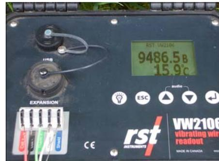
2. Switch on the unit and, where necessary, select range B
