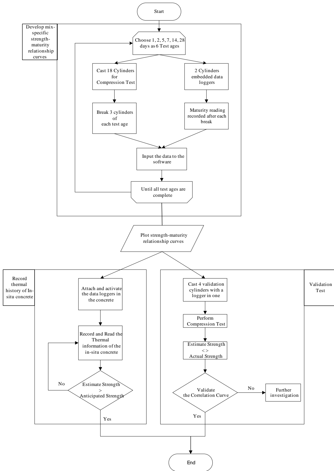
Figure 4-1 the maturity method process used in the pilot
