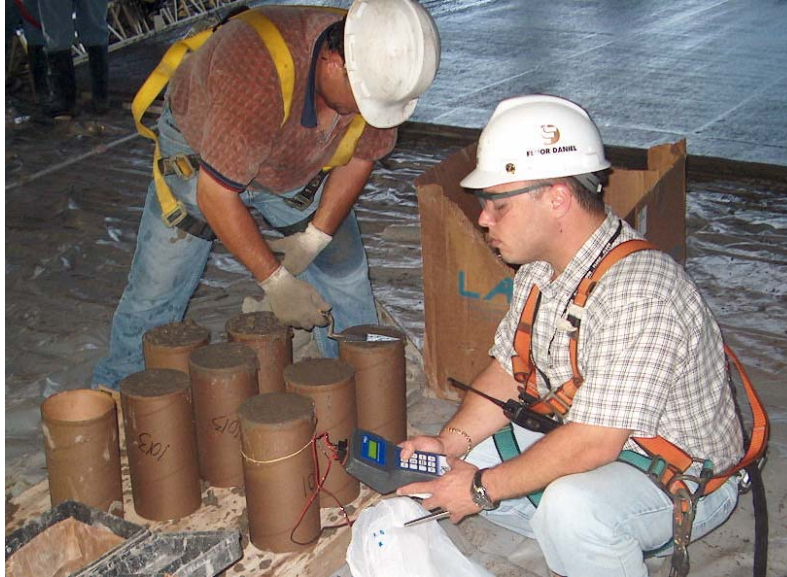
Figure 4-3 Validation Cylinder cast on site
