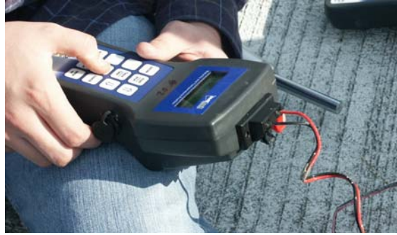
Figure 3-5: Connecting the IntelliRock reader to an embedded IntelliRock maturity logger
