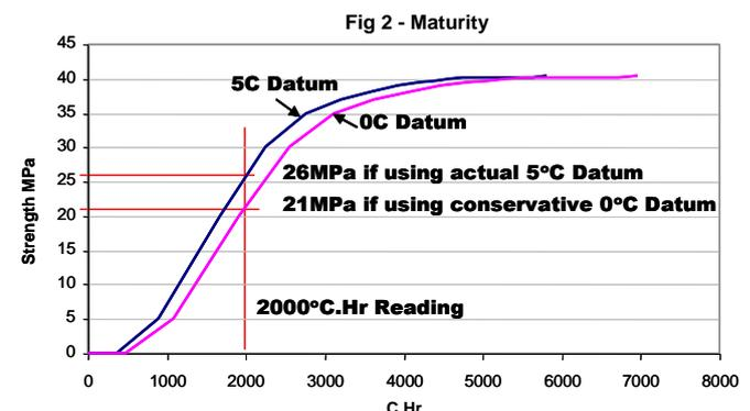
The strength predicted using the 0°C datum is 21 MPa compared to 26MPa using 5°C datum, i.e. the assumed 0°C datum gives a conservative strength assessment.
