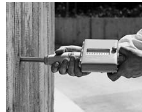
Fig. 2.2 Deploying the impact plunger (1) (model NR)
