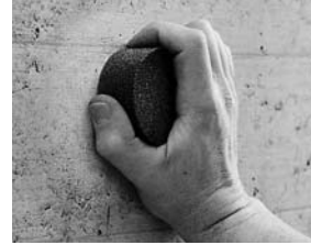
Fig. 2.1 Preparing the test surface
