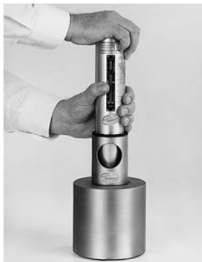
Fig. 3.1 Performance check of the concrete test hammer (model N/L shown)
