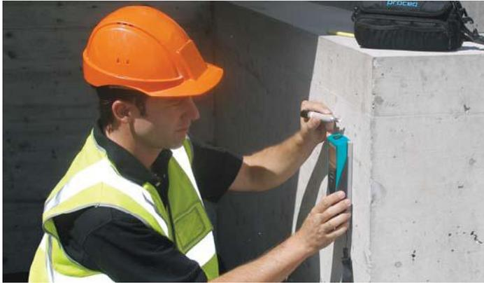
A rifle scope shows the position of the rebar beneath the instrument in real time. This is combined with red LED lights that illuminate when the bar is directly below the ProfoScope
