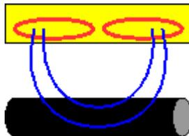
A pulse of current is sent (repeatedly) through a coil in the search head. This current tends to start up fairly gently (and is allowed to do so); see figure 1a. However, at the end
