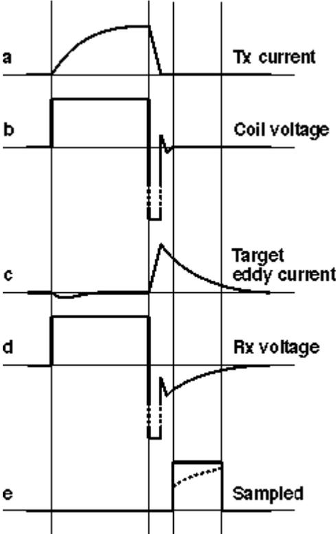
Figure 1: Coil Waveforms
