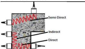
The Pundit PL-200 offers three methods of transmission. These can be seen in the image above. The method of transmission is determined by access to the concrete elements surfaces and the characteristic being tested.
