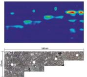
In this example a B-Scan of a concrete object containing steel pipes.
