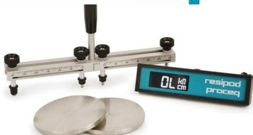
Surface resistivity measurement provides extremely useful information about the state of a concrete structure. Not only has it been proven to be directly linked to the likelihood of corrosion and the corrosion rate, recent studies have shown that there is a direct correlation between resistivity and chloride diffusion rate.
