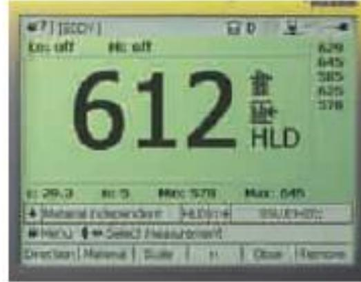
Modern electronics with power saving features provide for long operating life. The large LCD display always shows how the EQUOTIP is configured to test. Variable function keys allow for quick change of common test parameters, and the on screen hint line shows the other active control keys. The context sensitive help files give the operator quick access to the operating instructions with the press of a single button.
