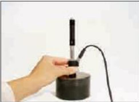
**3. Measure** Trigger the impact by pressing on the trigger button. The hardness value will be instantaneously displayed.
