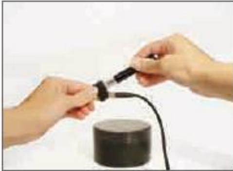
**2. Place-** Then place and hold the impact device on the surface of the test piece at the desired test point.
