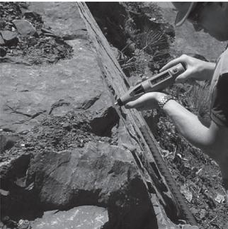
The number of test impacts required for a valid rebound number is defined in the guidelines. Unless you are using the weathering grade mode, this will typically be at least 10 impacts. The individual impacts should be separated by at least the width of the plunger. Ensure that the hammer is perpendicular to the test surface. Push the hammer against the surface at moderate speed until the impact is triggered.
