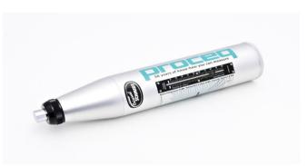
Rebound values are read from a dial and converted to compressive strength using the graphic above it.
