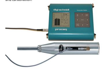
It comes with a number of pre-programmed correlation curves, allowing the user to select the most suitable for the mixture under test. All data and parameter may be transferred to a PC for further evaluation with the ProVista software.
