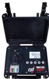
This unit allows a user to collect readings from a VW Sensor and Thermistor during installation or for short term jobs where a operator can check manually. With a switching box multiple VW system can be read one after the other.
