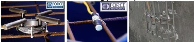
The CorroZoa will measure half-cell potential, corrosion current, and temperature. The unit can either be used manually or automated and left as a data logger.
