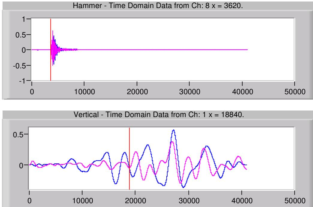
**Figure 2:** a. CS trigger data. b. CS up and down shear wave data (x-axis in microseconds, y-axis in output voltage). The vertical red lines mark the trigger time and the shear wave arrival time respectively.
