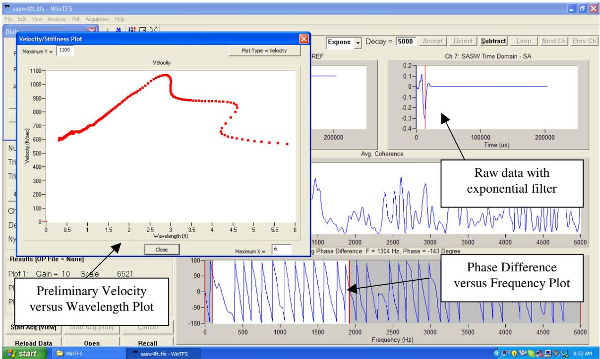
**Figure 3:** SASW raw data with exponential filter, phase difference plot with respect to frequency and primary velocity versus wavelength (depth) plot.
