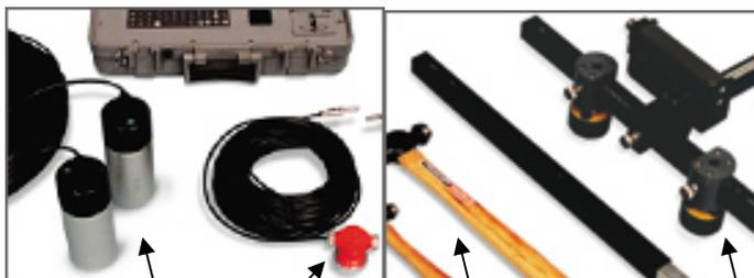
Accelerometer Geophone Hammer Fixed Receivers
