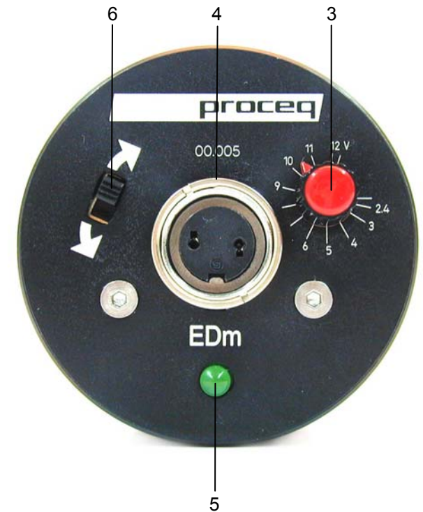
Fig. 4.01 Front plate of EDm motor drive
