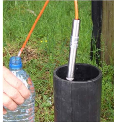
11. If necessary, coil up and feed the piezometer cable into the casing so that the drilling rig can be used to retract the casing. Ensure that there is enough slack cable to prevent the casing pulling the piezometer back up the borehole. ( This will have to be repeated whenever casing is to be raised or removed. ) When a section of casing is removed it will have to be slid along the cable or the cable passed through it.
