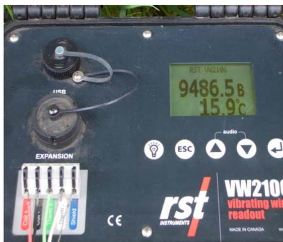
Prior to carrying out a 'Zero Reading' CHECK, ensure that the piezometers have been stored in a reasonably stable temperature for at least 30– 60 minutes.
