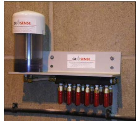
9. After the Settlement System has been buried/driven to the required depth, it can be connected to the reservoir.
