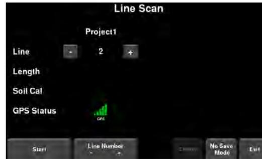
Press the **Start** button to begin collecting data. The screen will change to the data acquisition screen. As the system is pushed along a straight line, the collected GPR data scrolls onto the screen from the right and moves to the left.
